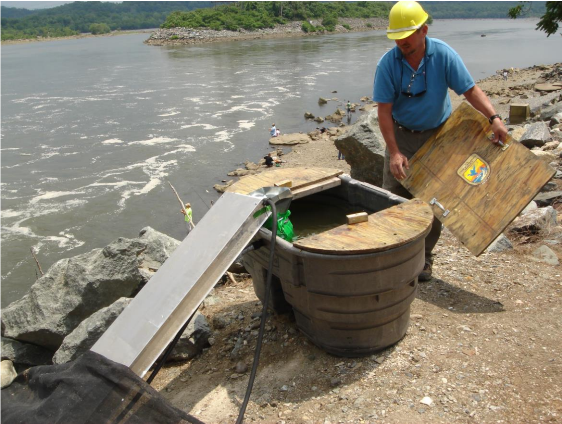
Figure 3. Cable tray emptying into a spat bag in the collection tank.
